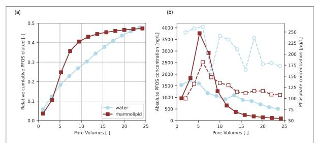
**Figure 1: (a)** Cumulative mass of perfluorooctane sulfonic acid (PFOS) eluted in the rhamnolipid and water flushing tests relative to the initial mass in the column. **(b)** Concentrations of PFOS (solid lines) and phosphate (dashed lines) in eluate of the water flushing test (blue circles) and the rhamnolipid flushing test (red squares).
