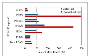
**Figure 3:** Percent mass of per- and polyfluoroalkyl (PFAS) compounds eluted from the column in the water and rhamnolipid flushing tests. *PFBA: perfluorobutanoic acid; PFBS: perfluorobutane sulfonate; PFHxA / PFHxS: perfluorohexanoic acid / perfluorohexane sulphonic acid; <i>PFOA: perfluorooctanoic acid; PFOS: perfluorooctane sulfonic acid.*
