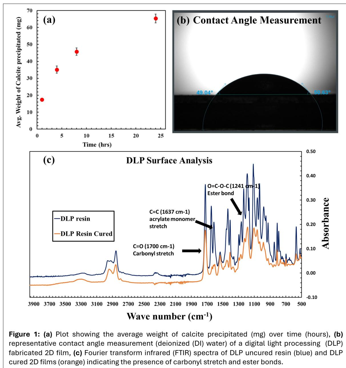
**Figure 1:** (a) Plot showing the average weight of calcite precipitated (mg) over time (hours), (b) representative contact angle measurement (deionized (DI) water) of a digital light processing (DLP) fabricated 2D film, (c) Fourier transform infrared (FTIR) spectra of DLP uncured resin (blue) and DLP cured 2D films (orange) indicating the presence of carbonyl stretch and ester bonds.
