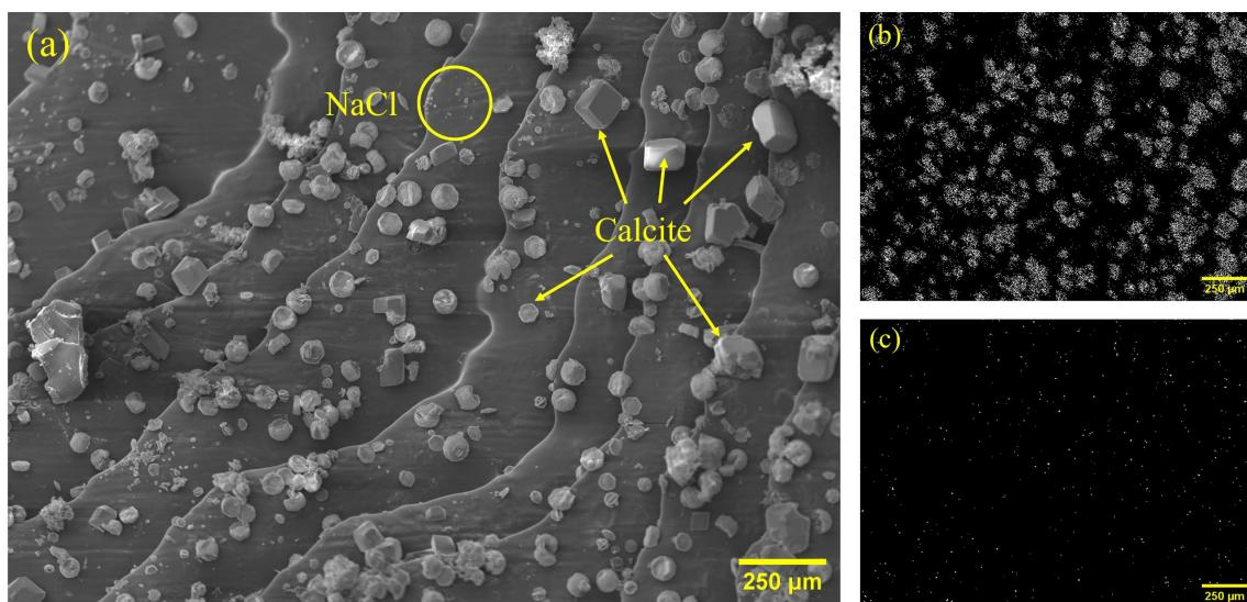
**Figure 4:** Secondary electron image of fracture surface after precipitation experiment showing (a) calcite and NaCl grains, and associated elemental maps of (b) calcium and (c) sodium.
