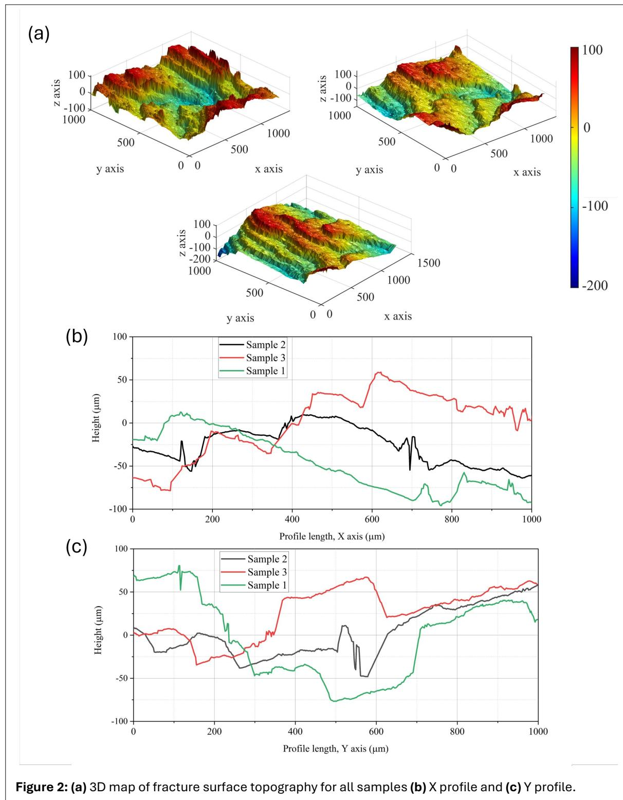
**Figure 2: (a)** 3D map of fracture surface topography for all samples **(b)** X profile and **(c)** Y profile.
