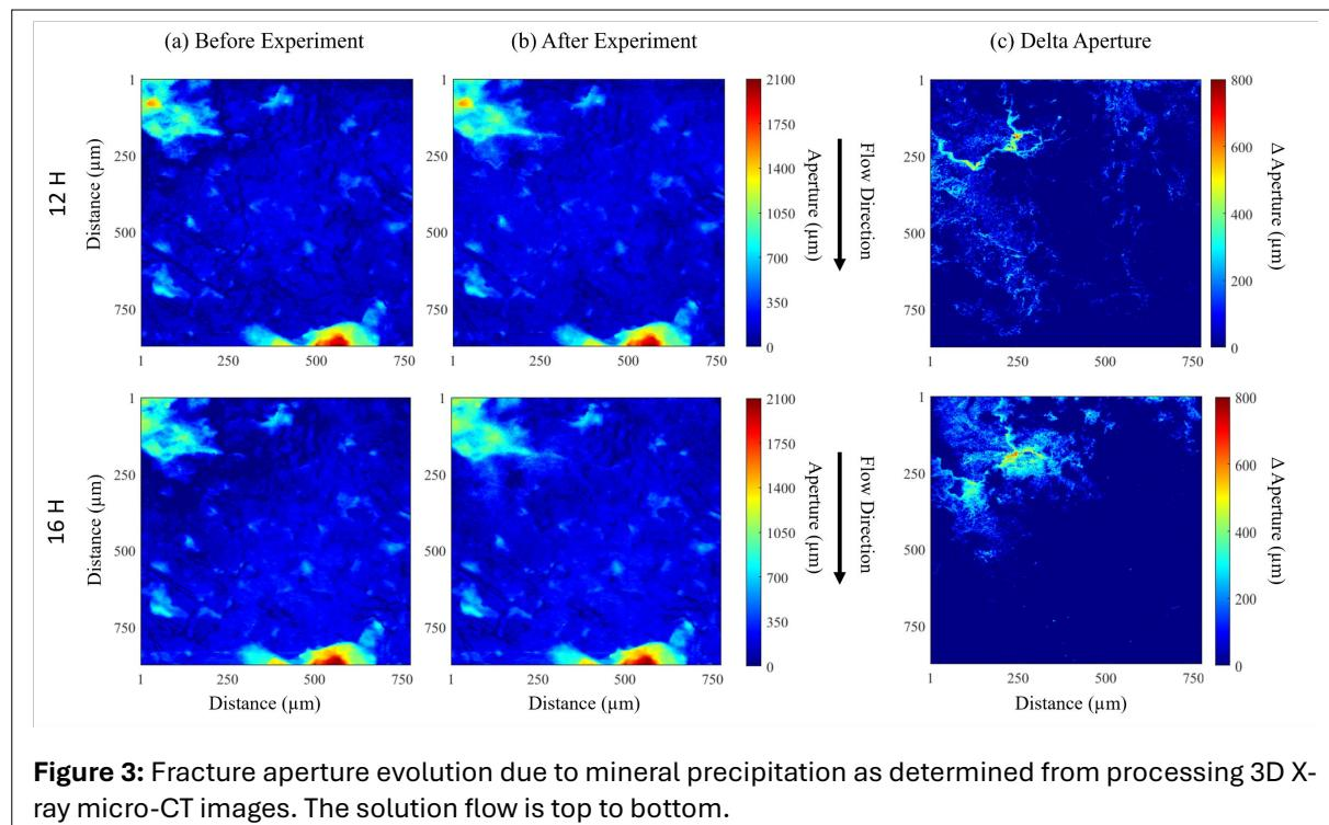
**Figure 3:** Fracture aperture evolution due to mineral precipitation as determined from processing 3D X-ray micro-CT images. The solution flow is top to bottom.
