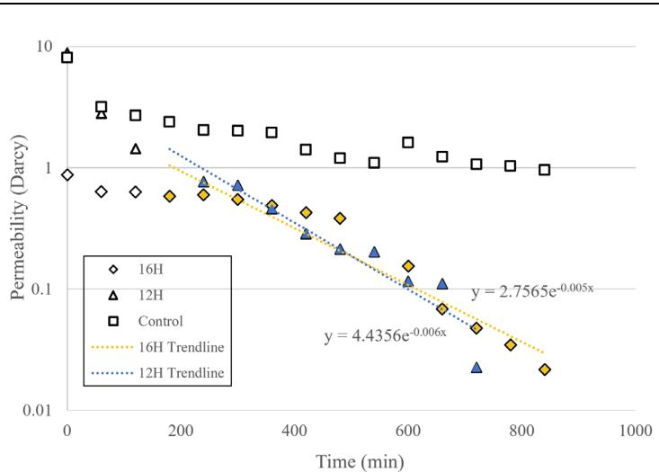
**Figure 5:** Experimental permeability evolution calculated from the differential pressure measurements. Data used for the trendlines are presented using colored markers: blue for the 12H experiment and yellow for the 16H experiment.
